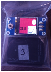
Fig. 2 The interaction device in action. Raspberry Pi Zero WH attached to TNTOR pocket-sized power bank
