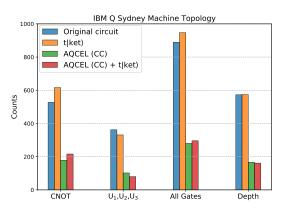
Fig. 4 Numbers of single-qubit  $(U_{1,2,3})$  gates, CNOT gates and the sum of the two as well as the depth of the one-branching step QPS circuit transpiled considering the ibmq\_sydney topology before and after the optimizations. The computational basis states with nonzero amplitudes at controlled gates are identified using classical calculation in the heuristic optimization step of AQCEL.
