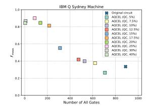
Fig. A-5 Fidelity  $F_{\text{meas}}$  versus the number of native gates for the one-branching step QPS circuit transpiled considering the ibmq\_sydney topology before and after optimization. The probabilities of observing various bitstrings in the control qubits are measured using the sydney in the heuristic optimization step, and the static thresholds of  $s_{\epsilon}^{f}$  are applied. These transpiled circuits are executed on the sydney to obtain the  $F_{\text{meas}}$ .
