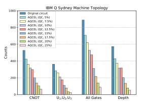
**Fig. A·3** Numbers of single-qubit  $(U_{1,2,3})$  gates, CNOT gates and the sum of the two as well as the depth of the one-branching step QPS circuit transpiled considering the ibmq\_sydney topology before and after optimization. The probabilities of observing various bitstrings in the control qubits are measured using the sydney in the heuristic optimization step, and the static cutoff thresholds of  $s_{\epsilon}^{f}$  are applied.
