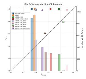
Fig. 7 Fidelities  $F_{\text{meas}}$  versus  $F_{\text{sim}}$  for the one-branching step QPS circuit transpiled considering the ibmq\_sydney topology before and after optimization under different schemes. These transpiled circuits are executed on the sydney to obtain the  $F_{\text{meas}}$  and a state-vector simulator to obtain the  $F_{\text{sim}}$ . The vertical bars represent the total number of gates in the circuits (gauged by the right-hand vertical axis).
