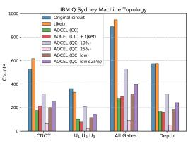
Fig. 6 Numbers of single-qubit  $(U_{1,2,3})$  gates, CNOT gates and the sum of the two as well as the depth of the one-branching step QPS circuit transpiled considering the ibmq\_sydney topology before and after optimization under different schemes.
