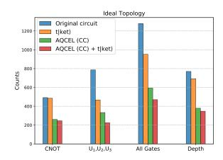
**Fig. 3** Numbers of single-qubit  $(U_{1,2,3})$  gates, CNOT gates and the sum of the two as well as the depth of the two-branching step QPS circuit decomposed into native gates before and after optimization. The computational basis states with nonzero amplitudes at controlled gates are identified using classical calculation in the heuristic optimization step of AQCEL.
