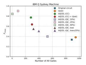
Fig. 5 Fidelity  $F_{\text{meas}}$  versus the number of native gates for the onebranching step QPS circuit transpiled considering the ibmq\_sydney topology before and after optimization under different schemes. These transpiled circuits are executed on the sydney to obtain the  $F_{\text{meas}}$ .
