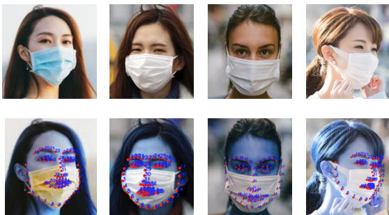
Fig. 4 Samples of face-mask-aware facial landmark detection of the GAN model in stage 1.
