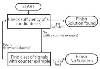
Figure 5 Overflow of iterative calculation of Signal Selection [2]
