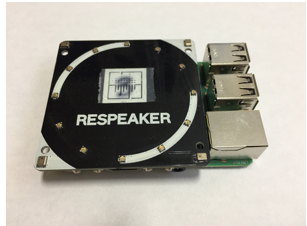
図6 測位デバイス:Raspberry Pi 3 Model B+ + ReSpeaker 4-Mic Array for Raspberry Pi
