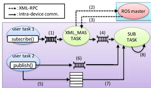
Fig. 8 Flow of intra-device communication.
