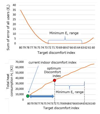
Fig. 2 Method to detect the optimum target discomfort index from the change of E<sub>s</sub> (top) and TDI (bottom) regarding environment discomfort index
