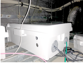
(a) Plastic box in which a BLE module is deployed
