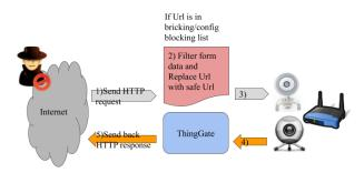
Figure 2 Filtering out unwanted traffic.
