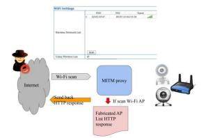
Figure 4 Protecting Wi-Fi information with ThingGate.
