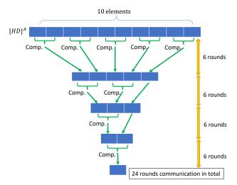
Fig. 3 Process of comparison part with n = 10, it requires 24 rounds of communications which is equal to  $6 \times \lceil \log_2 n \rceil$ .
