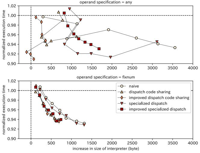
Fig. 14 Execution times and interpreter sizes for bitops-3bit-bits-in-byte.
