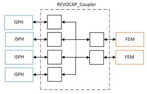
Fig. 1. The data communication by using REVOCAP Coupler
