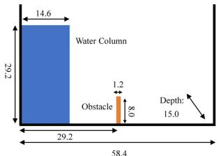
Fig. 2. A dam break problem with an elastic obstacle (unit: cm)
