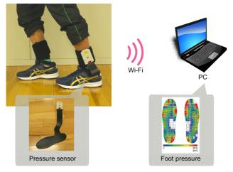
Fig. 1 System configuration.
