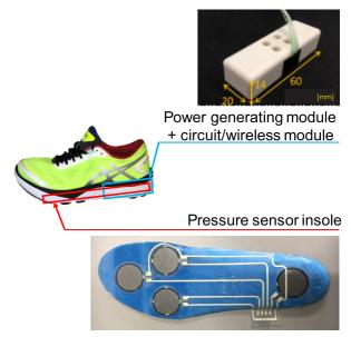
Fig. 10 Developed battery-free shoe device.
