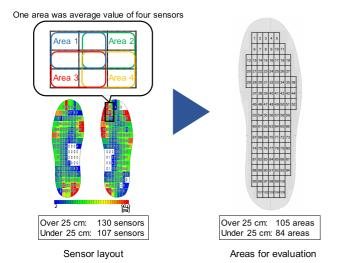
Fig. 3 Areas calculated from foot pressure sensors.
