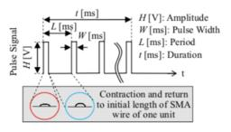
Fig. 2 Pulse signal for driving SMA wire.
