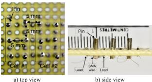
Fig. 1 Braille display with 2 Braille cells.
