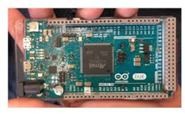
Fig.5 Arduino DUE.
