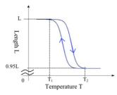
Fig. 3 Temperature Characteristics of SMA wire.
