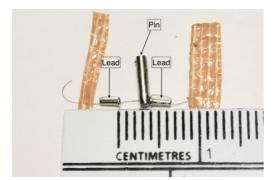
Fig. 4 Structure of SMA and pin.
