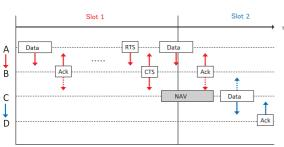
Fig. 4 Collision avoidance with RTS/CTS on slot boundaries.
