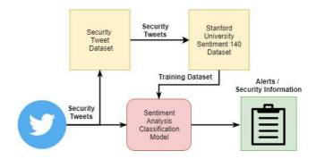
Figure 3: Diagram of overall system architecture
