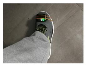
Fig. 1: Mount IMU on foot.
