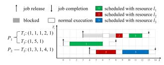
**Fig. 1** An example of blocking fractions.  $J_1$  arrives at  $t_3$ ,  $J_3$  at  $t_0$ , and  $J_2$  at  $t_4$ .  $R_1^{3,1,1}$  and  $R_1^{2,2,1}$  cause  $J_1$  to incur preemption delay and direct request delay, respectively.
