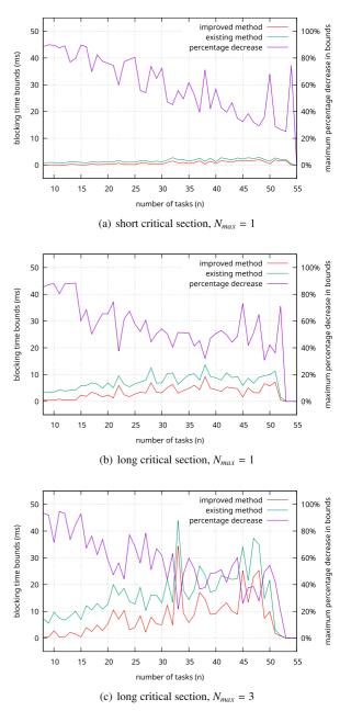
Fig. 5 Maximum percentage decrease in blocking time bounds under three combinations of parameters. We draw purple curves to show the maximum decrease between two methods. Yet red or green ones only represent the blocking time bounds in the case of maximum difference under the improved or existing method, respectively. They are not discussed independently.
