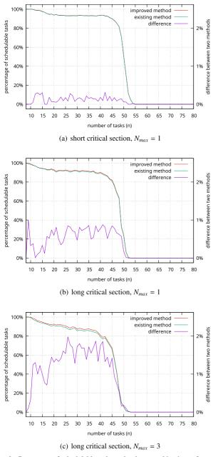
Fig. 6 Percentage of schedulable tasks under three combinations of parameters.
