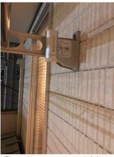
Fig. 5 Air temperature sensor in balcony
