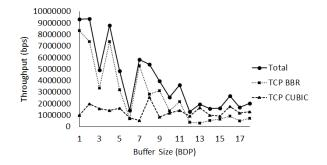
Figure 2: TCP BBR vs. TCP CUBIC [4]
