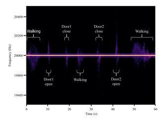
☑ 4 FFT spectrogram of front channel where the smartphone was placed 2.7 m away from the Door1 and 3.6 m away from the Door2 as shown in Figure 3
