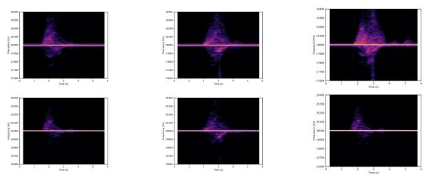
☑ 5 Spectrograms of a door opening where the door is situated (a) in front of the smartphone, (b) left side of the smartphone, (c) behind the smartphone. Spectrograms of the audio data from the front microphone is in the top row and the back microphone is in the bottom row.
