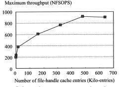
Fig. 15 Relation between maximum throughput and file-handle cache entries in the case of eightway X-NAS.
