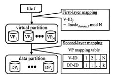
Fig. 4 File distribution by two-layer mapping.
