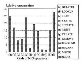
Fig. 10 Relative response time for NFS operations in the case of eight-way X-NAS.
