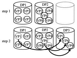
Fig. 5 Example of on-line reconfiguration.
