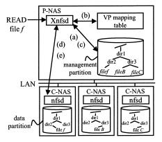
Fig. 3 Flow of READ operation.
