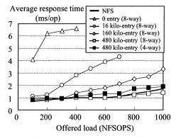
Fig. 11 Average response time of X-NAS with filehandle cache.
