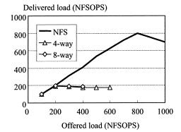
Fig. 9 Throughput of X-NAS without file-handle cache.
