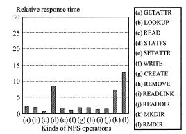
Fig. 13 Relative response time for NFS operations in the case of eight-way X-NAS.
