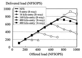
Fig. 12 Throughput of X-NAS with file-handle cache.
