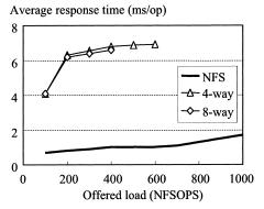
Fig. 8 Average response time of X-NAS without filehandle cache.
