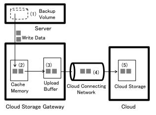
Figure 7 Cloud-based Data Backup System Model
