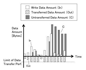
Figure 9 An Example of Untransferred Data Accumulation
