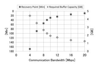
Figure 15 Performance Estimation by System Configuration
