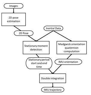
Fig. 5: Flow of the IMU trajectory estimation.
