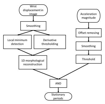
Fig. 6: Stationary moment detection.
