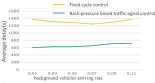
Fig 8. Comparison of the average vehicle delay under BP-TSC and fixed circle traffic signal control with fixed test traffic arrival rate.
