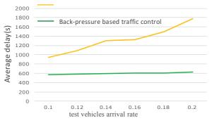
**Fig 7**. Comparison of the average vehicle delay under BP-TSC and fixed circle traffic signal control with fixed background traffic arrival rate.
