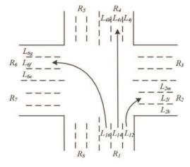
Fig. 1 Possible traffic movement from road  $R_I$  at junction  $J_i$ . enter  $L_{ij}$  from other roads, we define  $f_{ki_{2}ij}(t)$  to represent the number of vehicles moving from  $L_{ki}$  to  $L_{ij}$  in time slot t, so  $\sum_{k} f_{ki \rightarrow ij}(t)$  represents the total number of vehicles moving to  $L_{ij}$ in time slot t.
