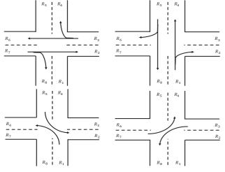
Fig. 2 Four typical phases through a junction.
