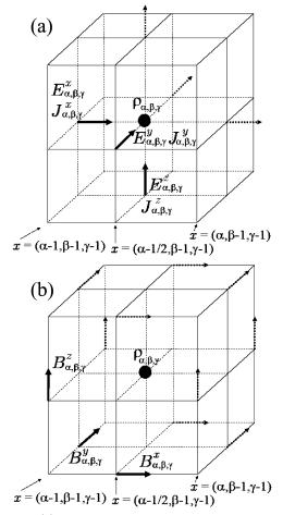
Fig. 1 (a) Locations where the electric field  $\boldsymbol{E}$ , the current density  $\boldsymbol{J}$ , and the charge density  $\rho$  are defined on a cell, and (b) those of the magnetic field  $\boldsymbol{B}$ .
