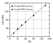
Fig. 7 Dependence of the computing performance (GFLOPS) on the total number of processors (PE). Here, the circles are the observed values in RUN1~3 which appear in Table 1, the triangles represent those in RUN4~6 which are presented in Table 2, and the solid line denotes the value of 12% of theoretical peak performance.
