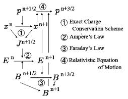
Fig. 2 Flow of calculation.
