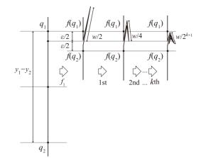
Fig. 12 Parallel shrink folding: reducing a horizontal strip down to small height.
