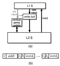
Fig. 4 Modified data path of L2 cache with writethrough L1 cache and write buffer in (a). An entry of write buffer in (b).
