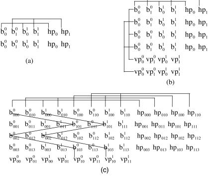
Fig. 3 Interleaving schemes to deal with MBEs. Bits are interleaved to tolerate horizontal MBEs in (a). Scheme in (b) tolerates horizontal & vertical MBEs but requires many vertical parity bits. Scheme in (c) can tolerate horizontal & vertical MBEs with fewer vertical parity bits.
