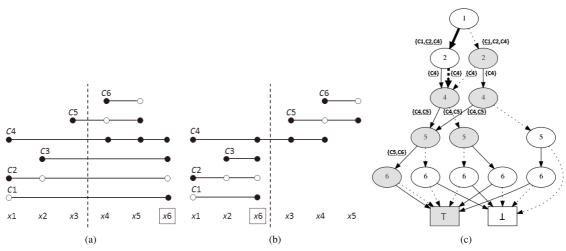
**Fig. 2** (a) CNF in original variable order, where  $x_6$  is dominated by  $x_1$  and  $x_2$ . (b) CNF in order determined by our method. (c) Constructed OBDD with our method. Nodes of label 3 are eliminated because 3-rd variable, i.e.,  $x_6$ , is dominated. Cutsets are used for equivalence test. Node labels mean a changed order of variables.
