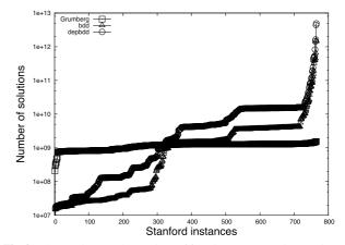
Fig. 3 Cactus plot w.r.t the numbers of found counterexamples, conducted with maximum node limit.
