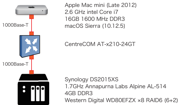
図 1 A diagram of benchmark setup for IOzone
