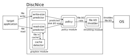
Fig. 5 Control flow in DiscNice.
