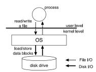
Fig. 4 Difference between file I/O and disk I/O.
