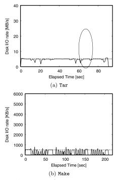
Fig. 14 Average disk I/O rate of tar and make with DiscNice.
