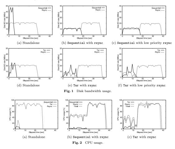
Figure 1 shows disk bandwidth usage in the experiment. We plotted a mean value within one second as disk I/O rate, based on a plotting scheme used by the other paper<sup>18</sup>). At first glance, the execution time of tar is different between Table 2 and Fig. 1. This is caused by Delayed Write, one of the OS features to improve system performance, as described in Section 2.2. Therefore, disk I/O requests are issued after tar finished its execution.
