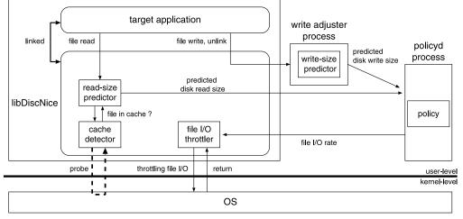
Fig. 9 DiscNice architecture.
