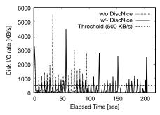
(c) Make (Disk I/O threshold is set to 500 KB/s)Fig. 13 Results of throttling macro-benchmark programs.
