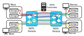
Figure 1: Overview of SDN-based Network Control Method
