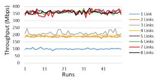
Figure 3: Throughput of each host (Link Aggregation)
