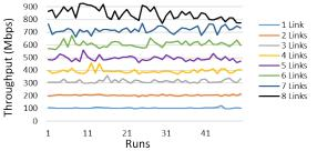
Figure 4: Throughput of each host (SDN-based Solution)
