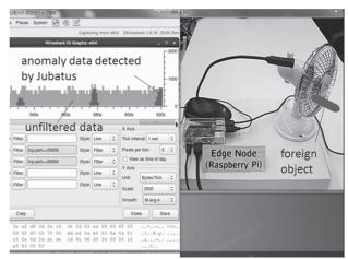
Fig. 2 Example application. (a) failure detection and shows an alert. (b) maintenance order to ERP. (c) comparing network bandwidth usage of unfiltered data and anomaly data detected by Jubatus.
