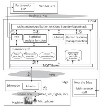
Fig. 1 Proposed maintenance platform architecture.
