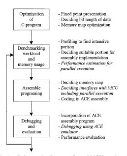
Fig. 7 Software development flow of MCU combined with ACE.
