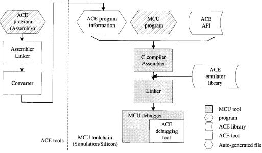
Fig. 8 Software development toolchain of MCU with ACE.
