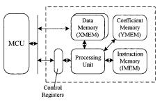
Fig. 1 Typical hardware structure of ACE combined with MCU.
