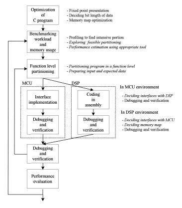
Fig. 6 Software development flow of MCU combined with general-purpose DSP.
