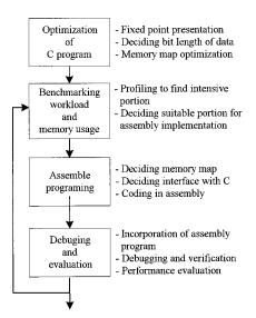
**Fig. 5** Software development flow of conventional MCU.
