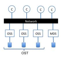
Fig. 1 Diagram of a typical cluster with luster nodes.
