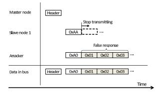
Fig. 4 Time chart of data from master node, slave node 1, attacker, and data in bus when a collision occurs between the first byte of responses. The value of the first byte in bus will be 0xA0 (= 0xAA & 0xA0).
