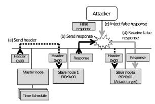
Fig. 3 Attacker induces collision between response sent from slave node 1 and false response.
