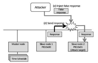
Fig. 6 After collision between headers, attacker injects a false response.
