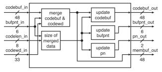
**Fig. 6** Circuit for packing codebuf register and updating bufpnt register, pn register, and membuf register in encoding.
