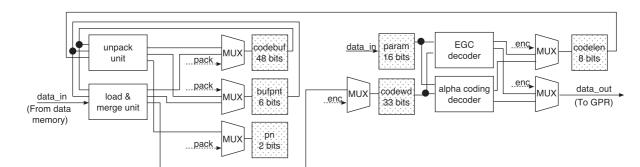
Fig. 7 Dedicated circuits and registers for decompression.
