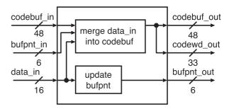
Fig. 9 Circuit for merging data from data memory to codebuf register and updating bufpnt register in decoding.
