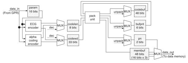
Fig. 5 Dedicated circuits and registers for compression.
