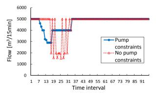
**Fig. 5** Example of optimal water distribution from a pump station over 96 time intervals.
