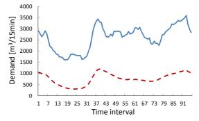
Fig. 3 Maximum values (solid line) and mean values (dashed line) for water demand at all the demand points every 15 minutes from 22:00 in a typical day.
