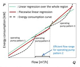
Fig. 2 Conceptual diagram of the energy consumption curve developed by pump modeling (dashed line) and two approximations by the linear regression over the whole flow range (dotted line) and the piecewise linear regression over each of the efficient flow ranges (solid line).
