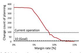
Fig. 4 Relation between the margin rate of gross water supply quantity for the total amount of water demand and the change count of the original plan with RO.
