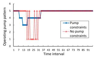
Fig. 6 Example of optimal pump operations at a pump station over 96 time intervals.
