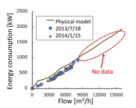
Fig. 1 Comparison between the energy consumption curve based on the physical model and past actual values at a typical pump station.
