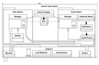
Fig. 2 Broker Class Model
