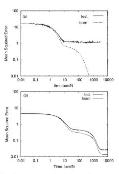
Fig. 2 Effect of dropout. (a) is the learning curve of SGD, and (b) is that of dropout learning.
