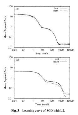
A comparison between Fig. 3 and Fig. 7(b) reveals that the residual error of dropout learning was almost the same as that of the SGD with L2 regularization. Therefore, the regularization effort of dropout learning is the same as the L2. Note that for the SGD with L2, we must choose  $\alpha$  in trials; however, dropout learning has no tuning parameter.
