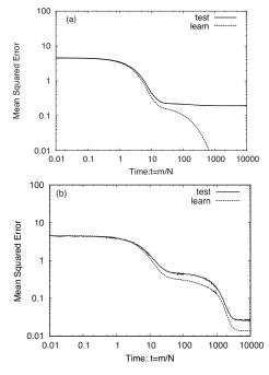
Fig. 7 Results of comparison between dropout and ensemble learning. (a) is ensemble learning of two networks, and (b) is dropout with respect to p = 0.5.
