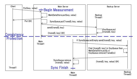
Fig. 3 Measurement point for our proposed method where key is separated from its value
