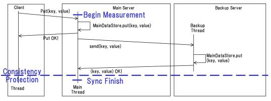
Fig. 4 Measurement point for traiditional approach where key is transmitted together with its value
