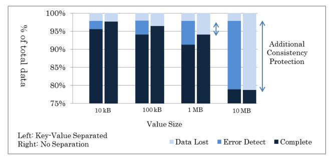
Fig. 8 Additional consistency protection obtained from key-value separation
