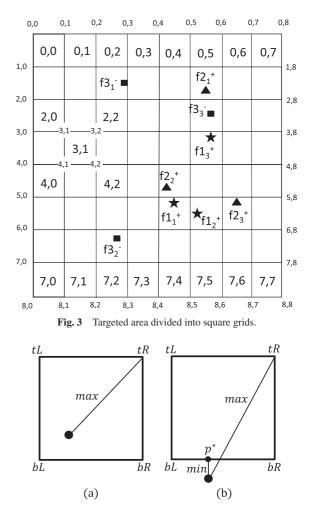
Fig. 4 Min. and Max. distance between grid and point.
