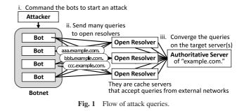
resolvers simultaneously query the authoritative servers, sharply increasing the load of the target servers. Further, the load on the cache servers, especially upstream ISP servers referred by bad home routers, also increases since recursive queries require more
