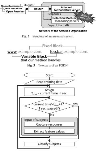
Fig. 4 Flowchart of the detection algorithm (on-the-fly detection mode).
