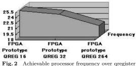
**Fig. 2** Achievable processor frequency over gregister size variation.
