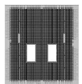
Fig. 1 Floorplan of the placed and routed PQPpfB processor core. The pipeline stages have been placed from the top right to the lower left corner of the target Stratix EP1S25F1020C5 FPGA device.
