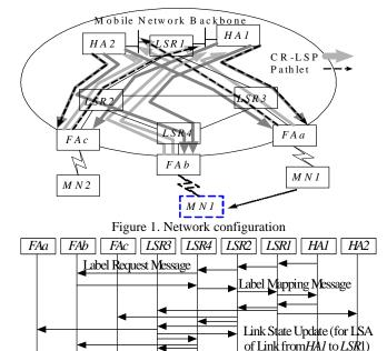
Figure 2. Sequence of establishing CR-LSP from HA1 to FAb
