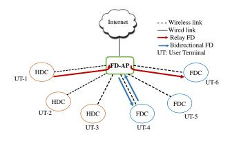
Figure 1: Structure of a full-duplex WLAN.
