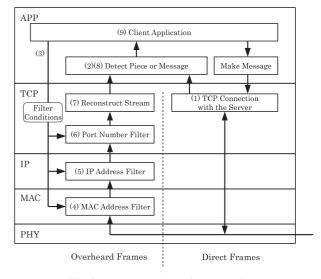
Fig. 3 Control procedures for overhearing.
