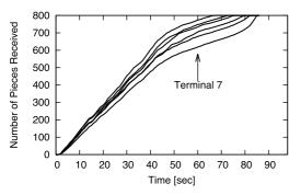
**Fig. 6** Cumulative number of pieces received for each terminal (Method B, Simultaneous start).
