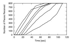
Fig. 9 Cumulative number of pieces received for each terminal (Method A, Sequential start).
