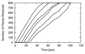
Fig. 10 Cumulative number of pieces received for each terminal (Method B, Sequential start).
