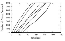
Fig. 11 Cumulative number of pieces received for each terminal (Method C, Sequential start).
