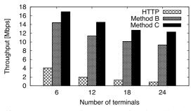
Fig. 12 Average throughput for the number of terminals (Simultaneous start).
