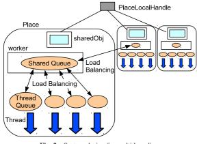
Fig. 2 System design for multithreading.
