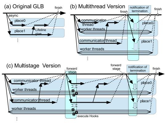
Fig. 5 Termination detection of tasks and stage migration.
