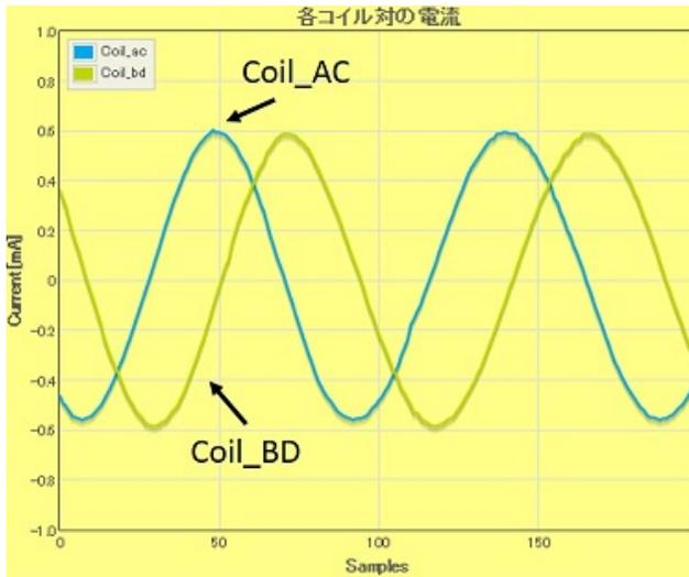
Fig. 12. Current waveforms of reverse rotation (High Speed).
