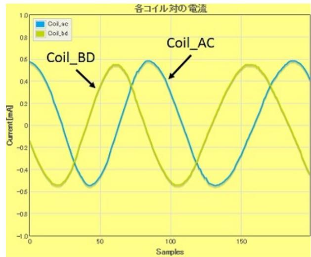
Fig. 11. Current waveforms of normal rotation (High Speed).
