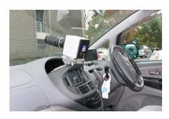
Fig. 4. High-speed camera used as receiver
