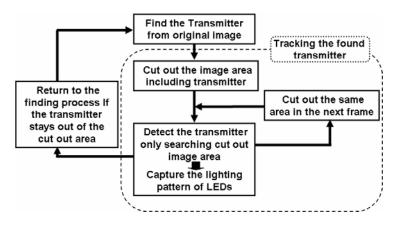
Fig. 5. The main image processing steps for the receiver
