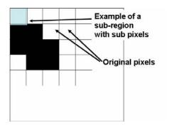
Fig. 11. Sub-regional division of transmitter image area using sub-pixels
